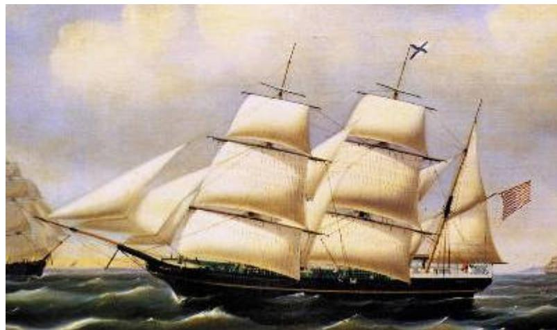
The Bremen bark *HANSA* was built at Vegesack/Fähr by H[ermann] F[riedrich] Ulrichs, for the Bremen firm of B. Grovermann & Co, and was launched on 14 September 1852. 153 Commerzlasten / 343 tons register; 36,2 x 8,2 x 4,1 meters (length x beam x depth of hold). Her masters were, in turn, August Brinkama and Georg Jaburg, both of Vegesack, and Peter Heyn, Ad. Büttner, and H. C. L. Riefe, all of Bremen.
